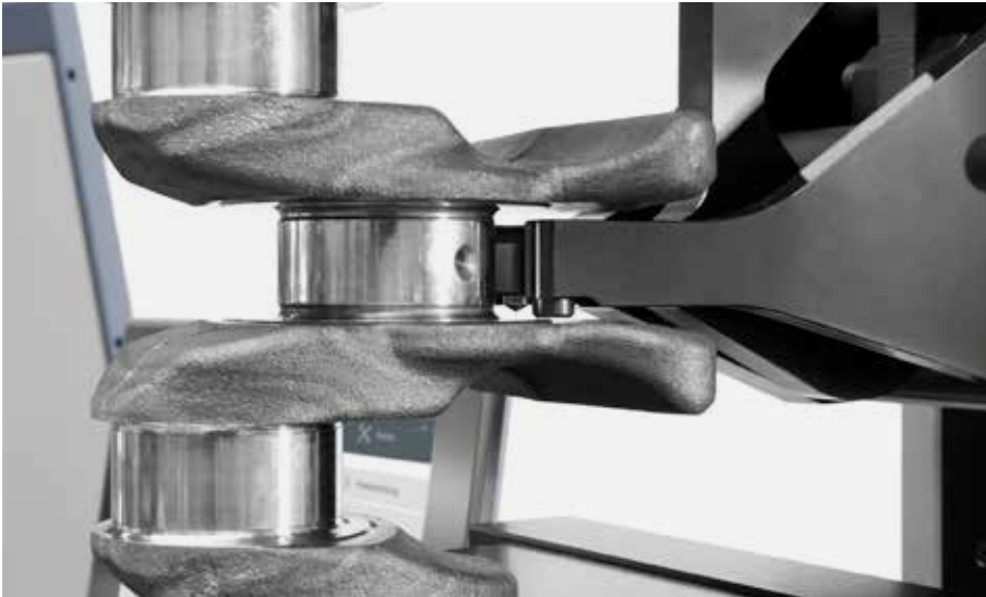
INDENTOR EXTENSION FOR HARD-TO-REACH TEST LOCATIONS
