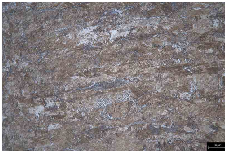
The microstructure of the welding joint after etching with 3% nitric acid – 200 x
