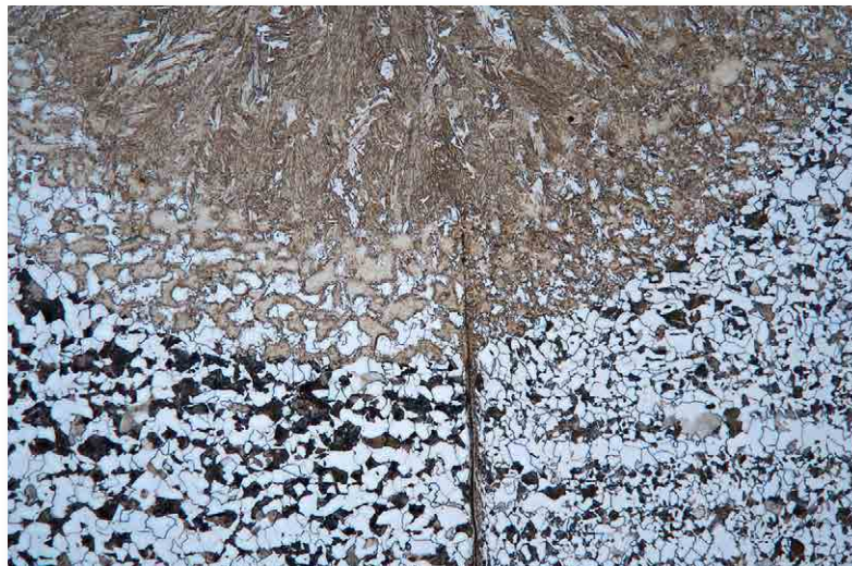
TIG welding zone and heat-affected zone after etching with 3% nitric acid – 200 x
