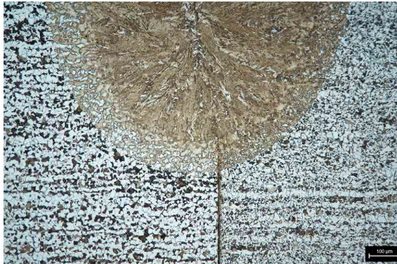
TIG welding zone and heat-affected zone after etching with 3% nitric acid – 100 x
