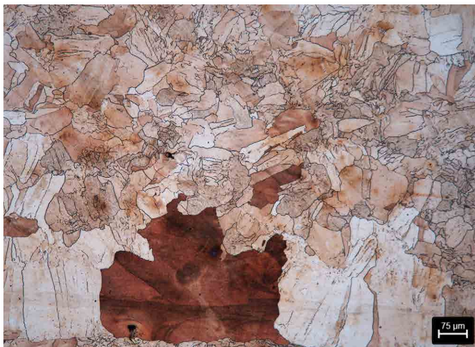
Copper sample after etching with etchant Copper A - 100x
