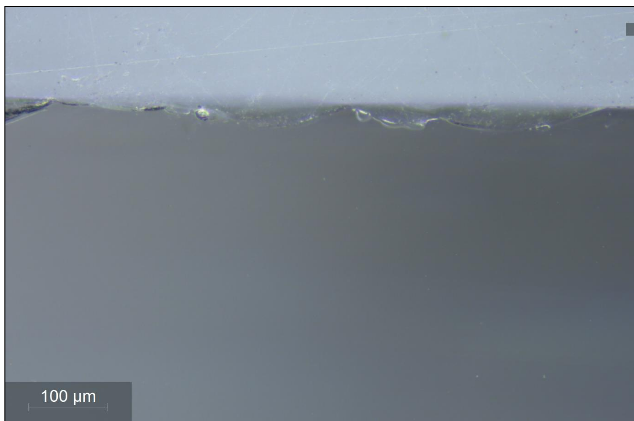
Figure 5: Glass surface after polishing with GAMMA and 3 µm – edge area with darkfield -100 x.
