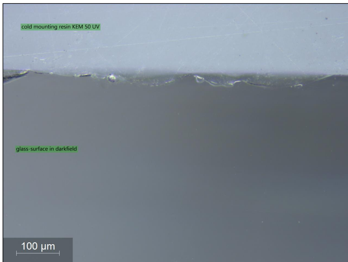
Figure 6: Glass surface after polishing with GAMMA and 3 µm – edge area with darkfield - 100 x.
