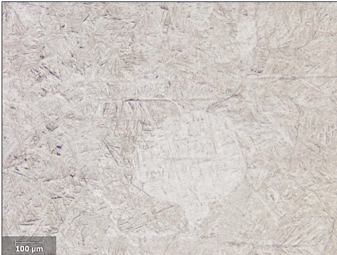
Figure 10: Sample 2 - screw head area after fine-polishing and etching with Kroll for 30 s – 50 x.
