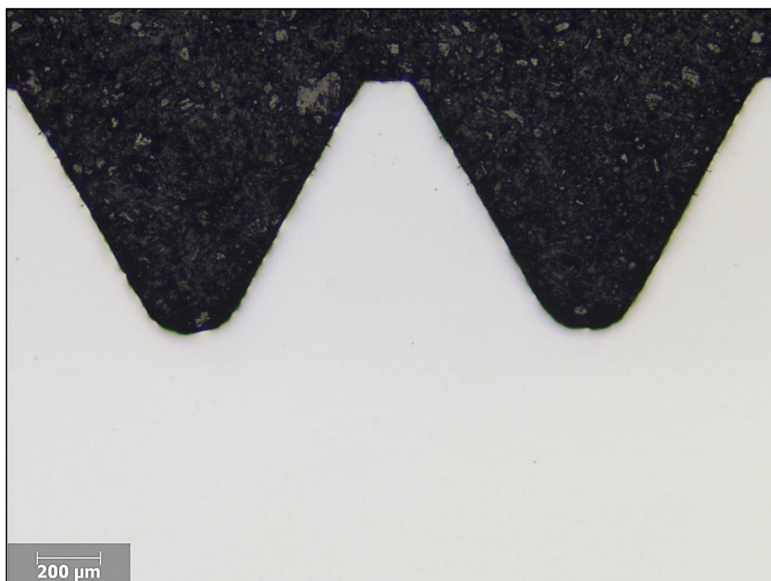
Figure 5: Sample 1 - thread area after fine-polishing – 50 x.
