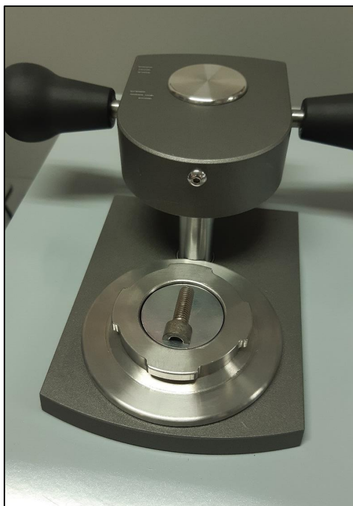
Figure 4: Overview of the mounting process with Opal 410.
