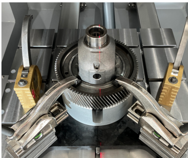
Special clamping device with sample adapter
