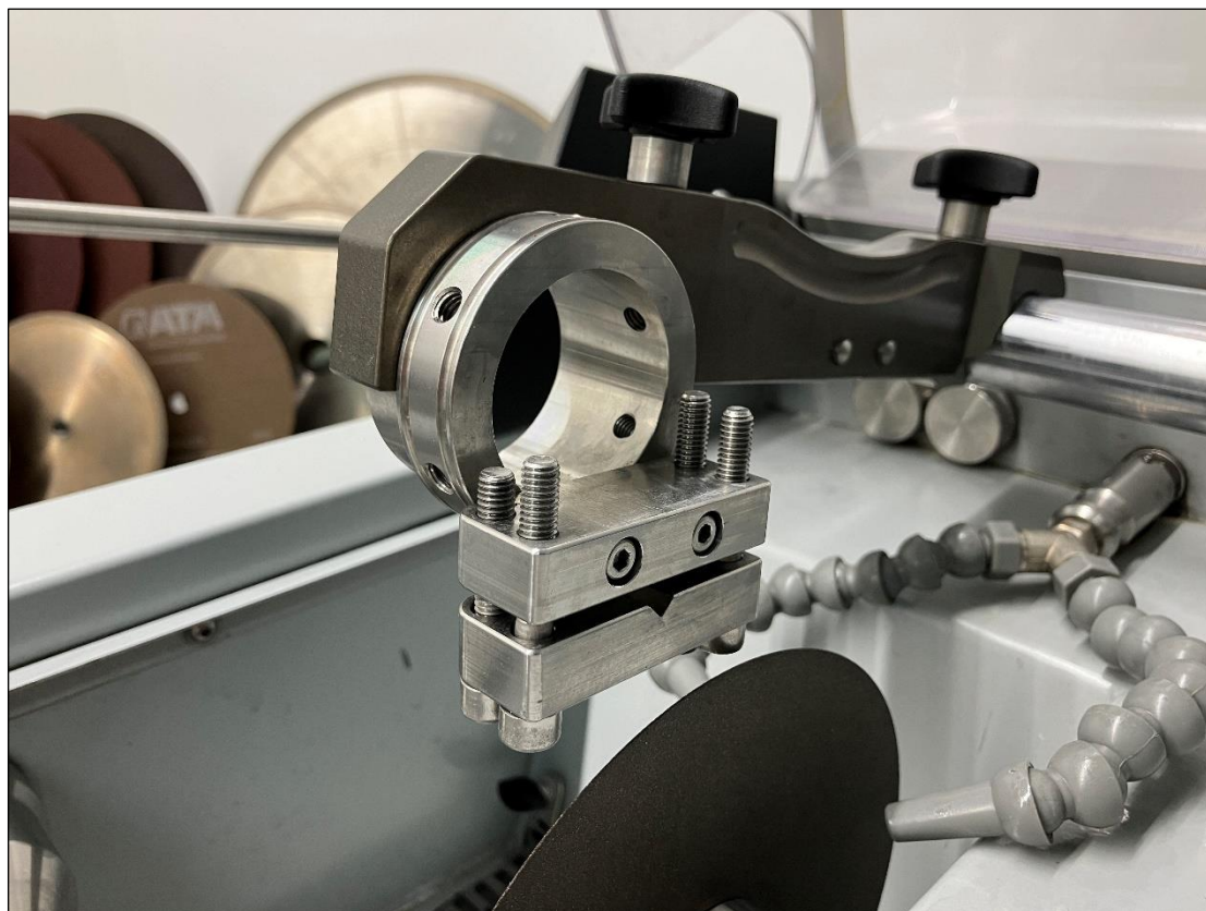
Figure 7: Overview of recommended clamping tool for graphite plate with surface coating.
