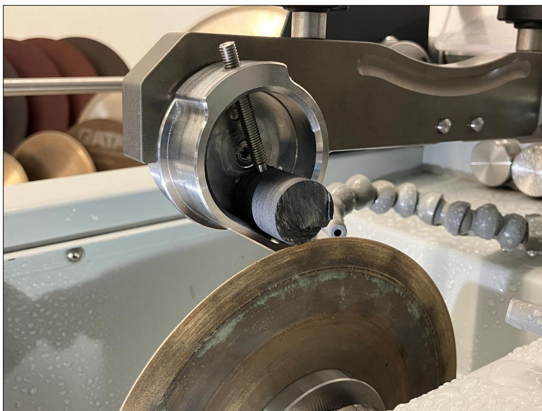
Figure 4: Overview of graphite cylinder with clamping tool clamping arm L + drop shape sample holder.
