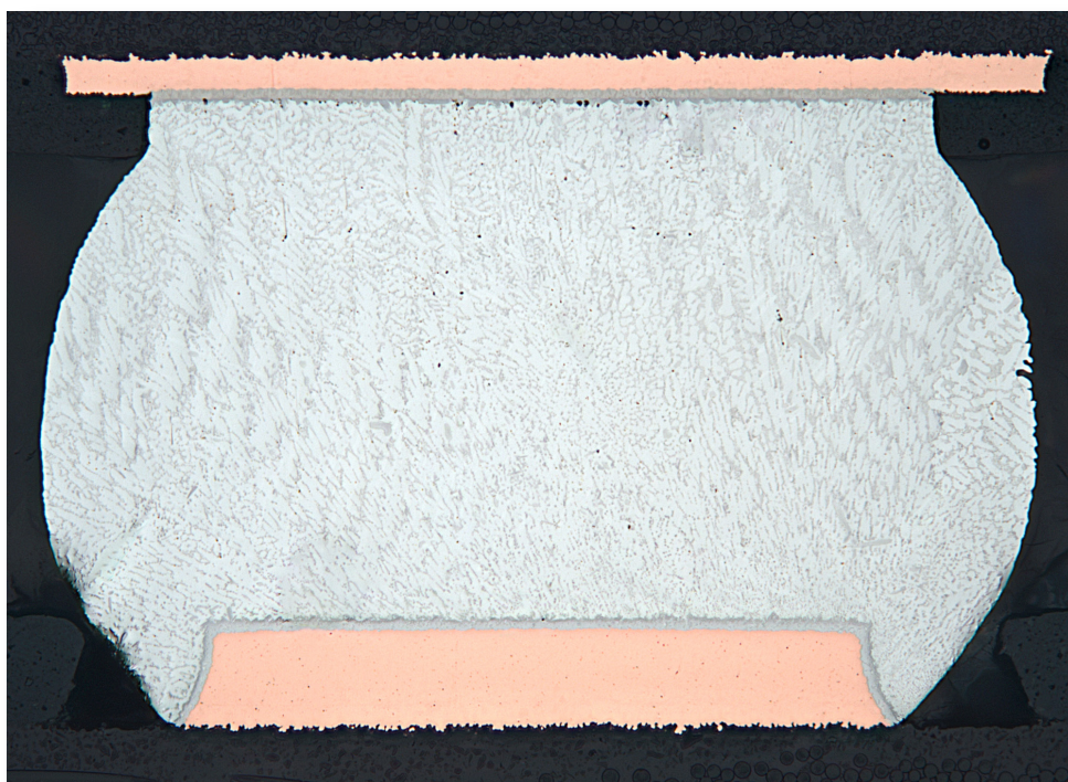
Solder ball without errors - 200:1
