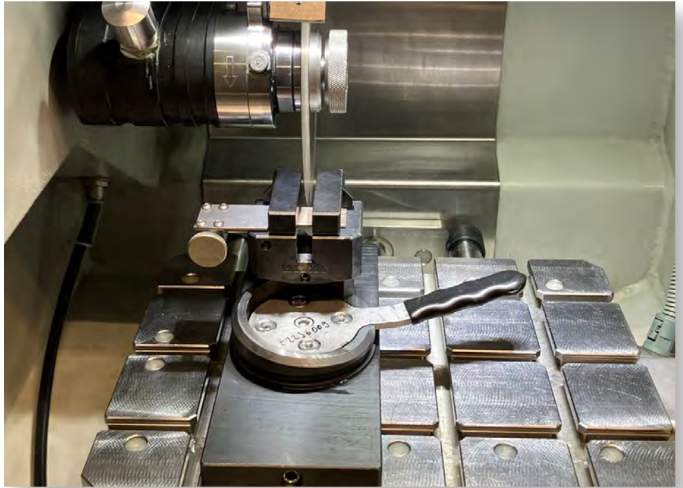
Clamping tool "Vertical Vice Single" (RECOMMENDATION 1)
