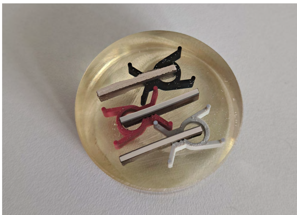
The sample after mounting
