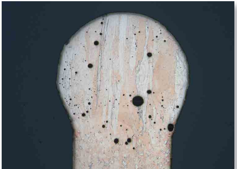
The weld seam after etching with Klemm II - 25 x
