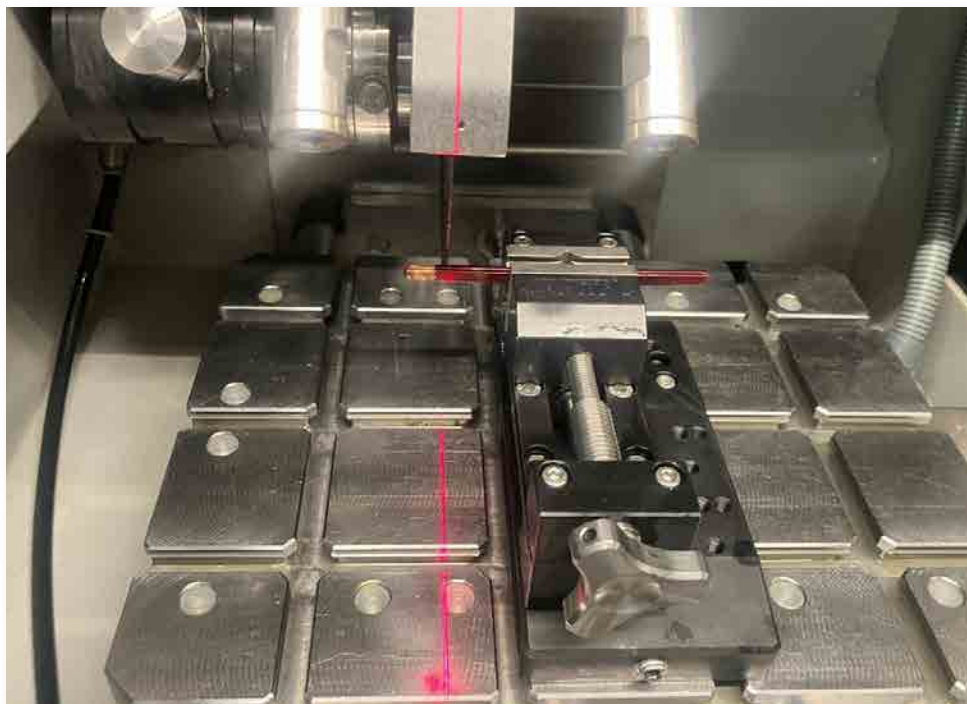
The sample clamped in the clamping tool
