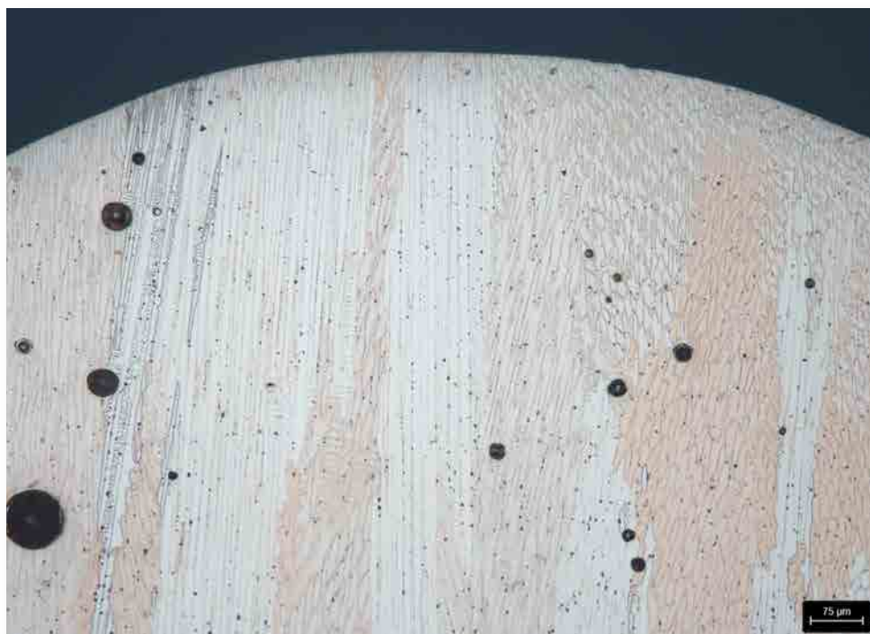
The weld seam after etching with Klemm II - 100 x
