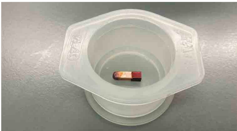
The sample in the cold mounting mold
