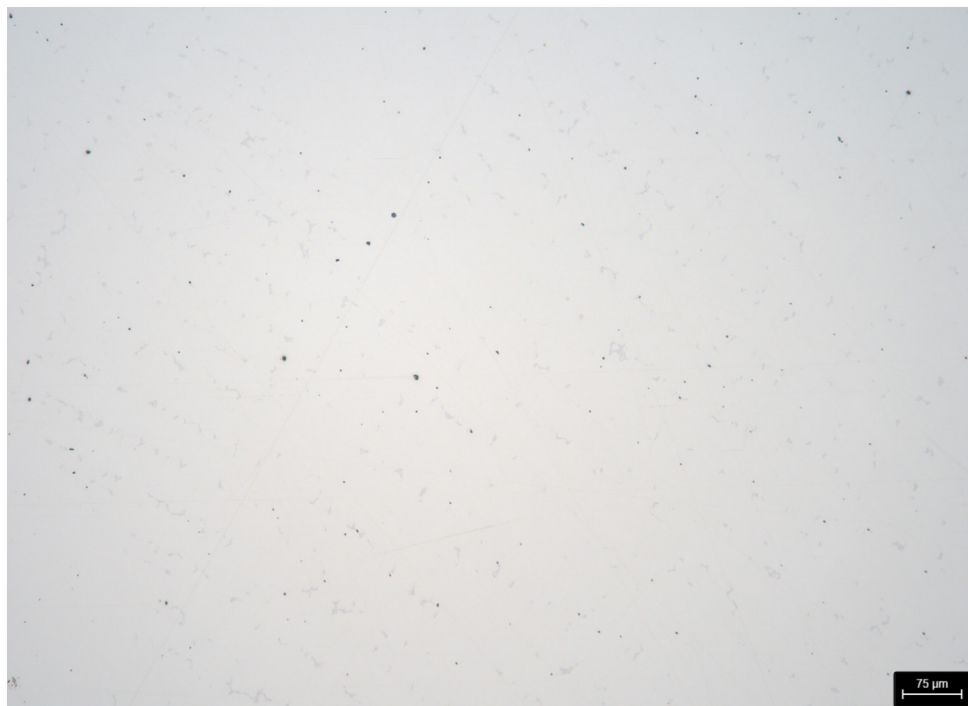
The CoCrMo cast alloy structure under the light microscope - 100 : 1 (unetched)
