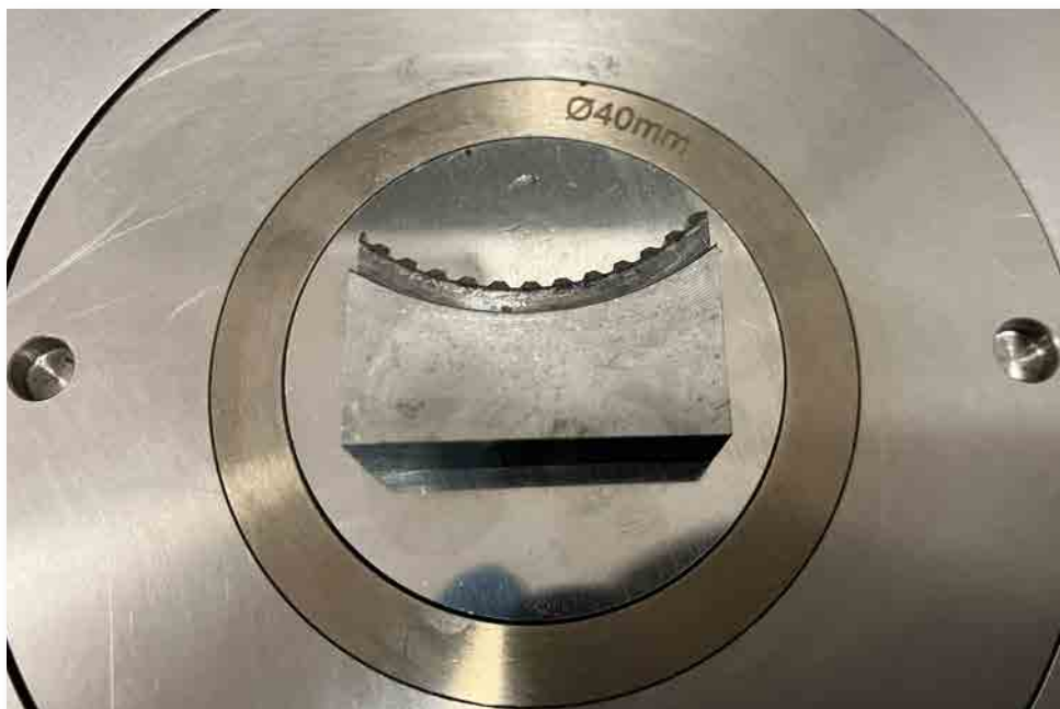
The cut samples on the piston of the hot mounting press
