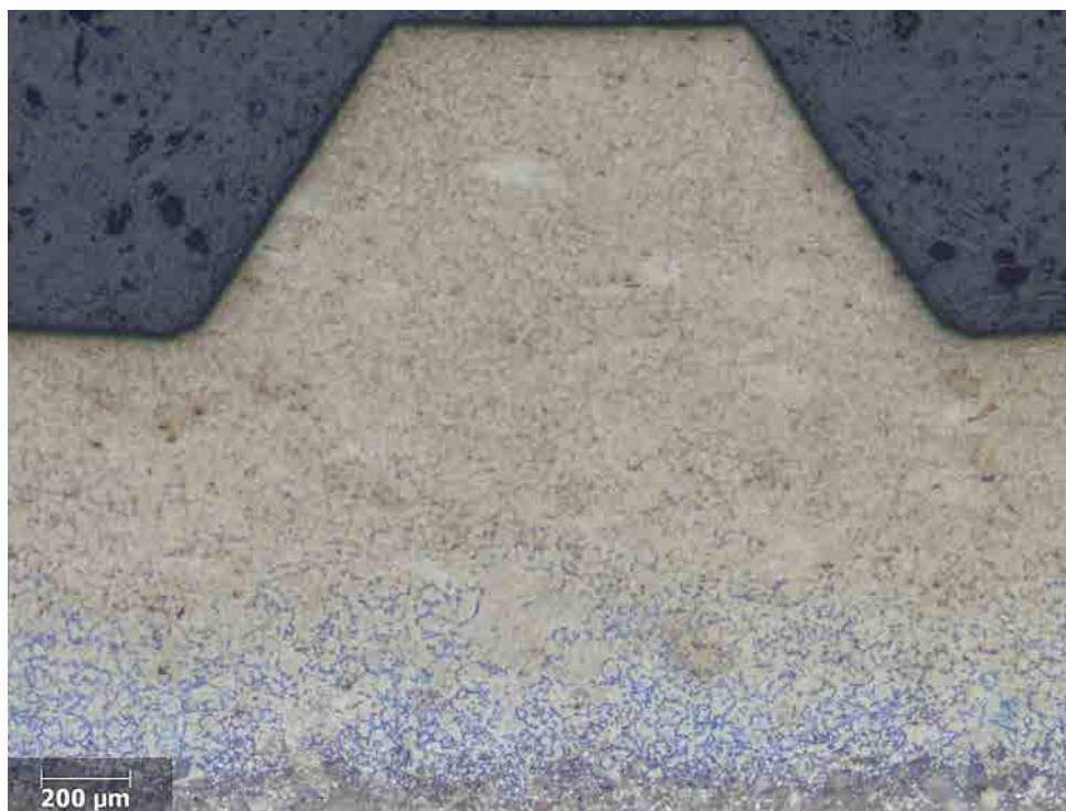
The microstructure on the edge region after etching under optical microscope- 25:1
