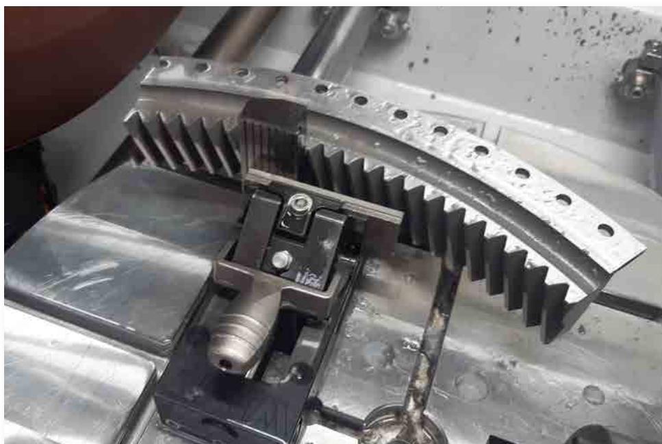
Clamping of the gear rack in Qcut 600 BOT
