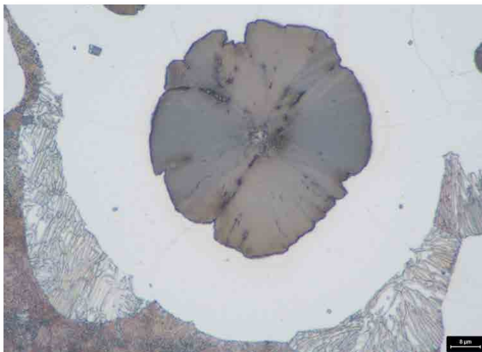
A spheroidal graphite particle after polishing and etching – 1000:1.
