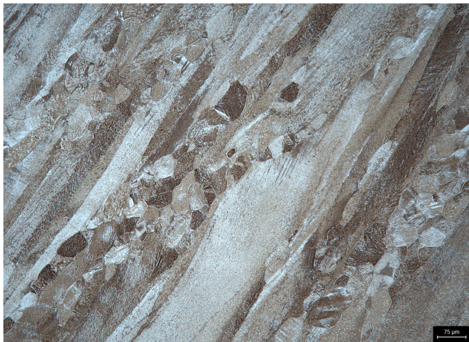
The microstructure of titanium alloy under the light microscope – 100:1
