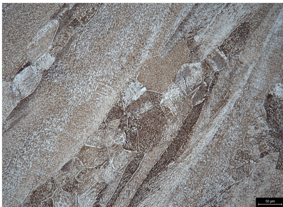
The microstructure of titanium alloy under the light microscope – 200:1
