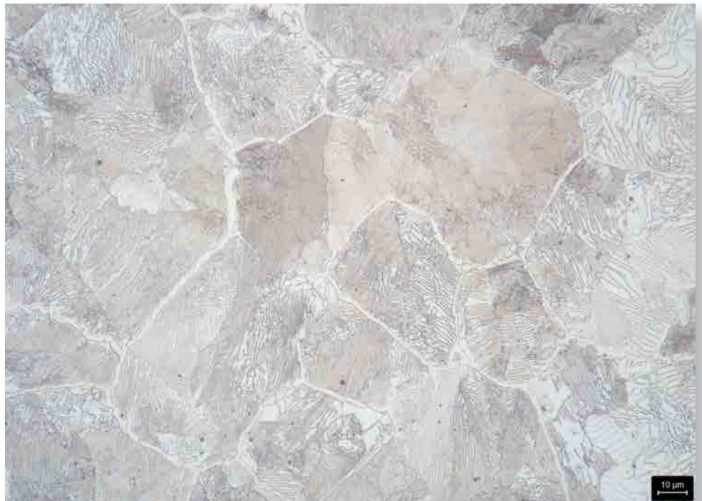
The microstructure containing perlite and secondary cementite after etching- 500:1
