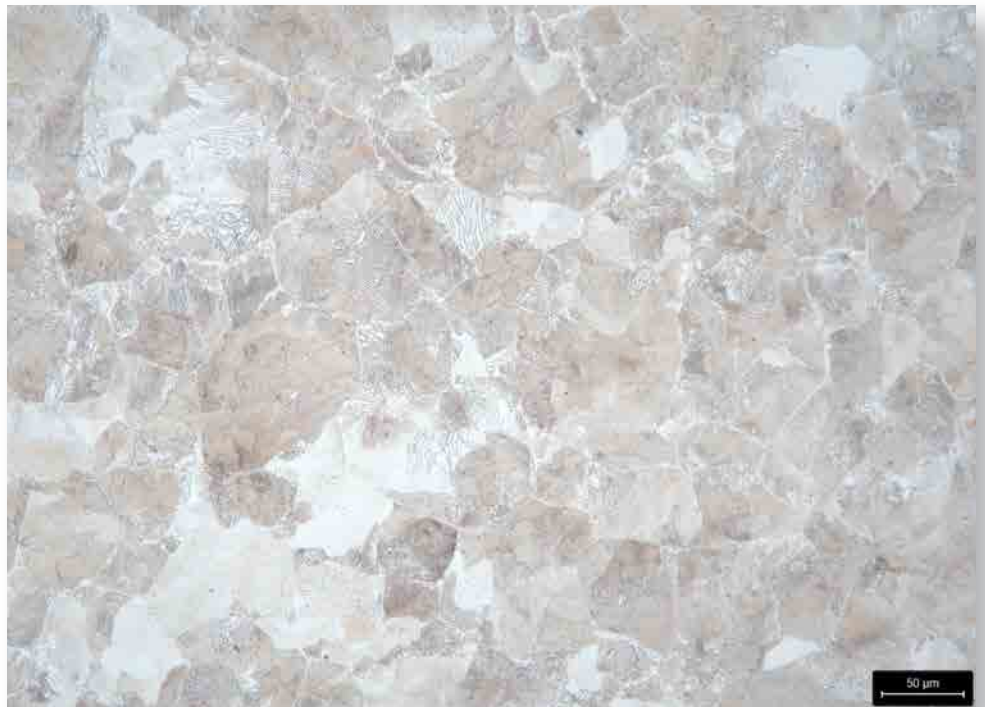
The microstructure containing perlite and secondary cementite after etching- 200:1
