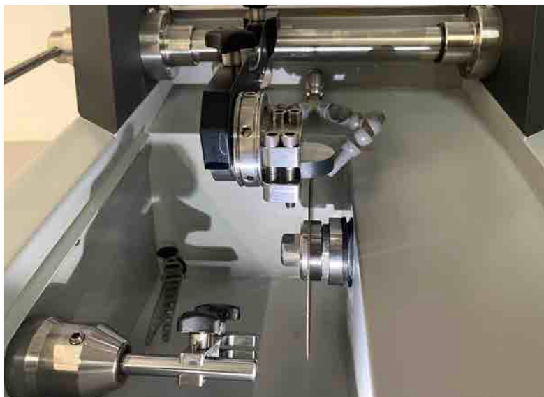
The clamping set-up in the cut-off machine Qcut 150 A
