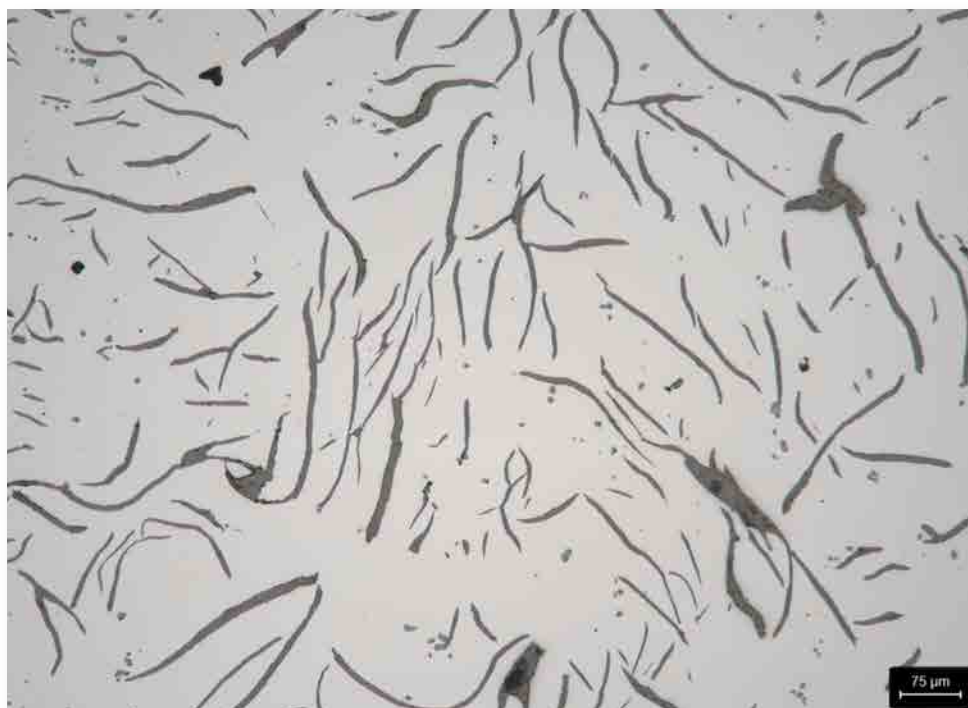
The microstructure of GJL after the 1 \mu\text{m} step under the microscope (100:1)
