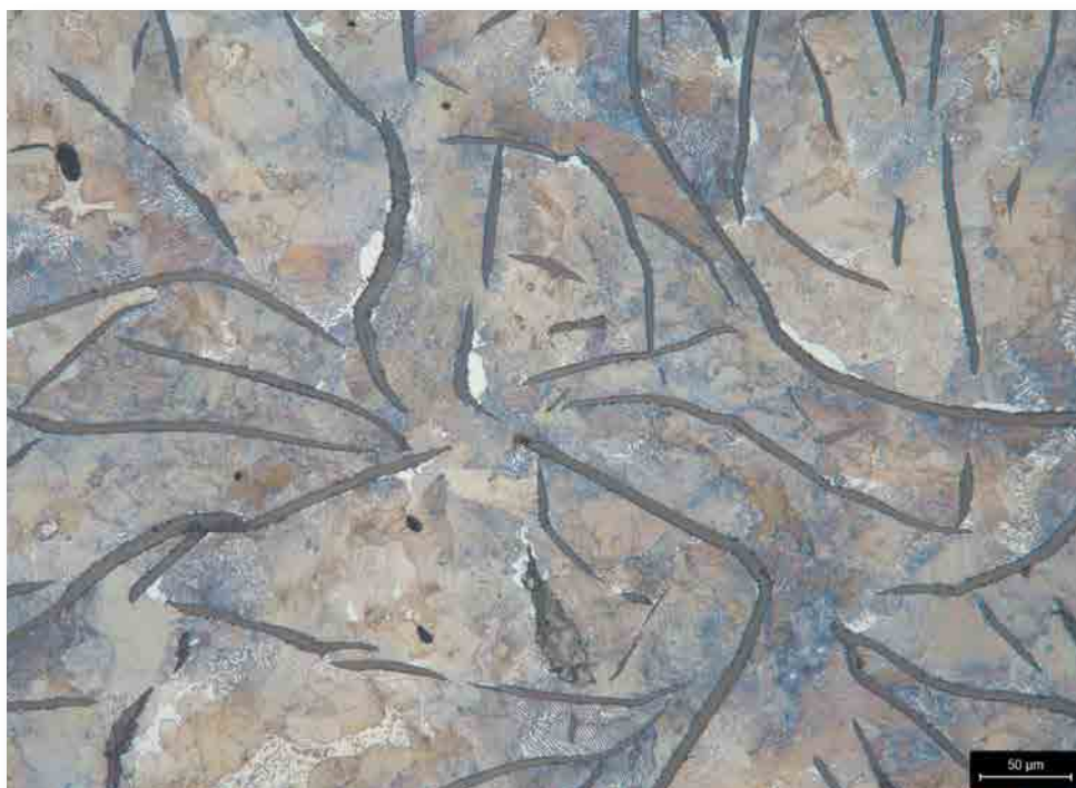
The microstructure of GJL after etching under the microscope (200:1)
