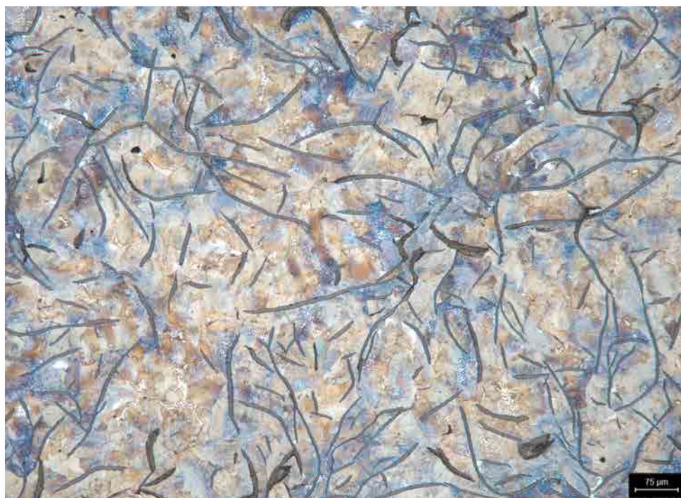
The microstructure of GJL after etching under the microscope (100:1)
