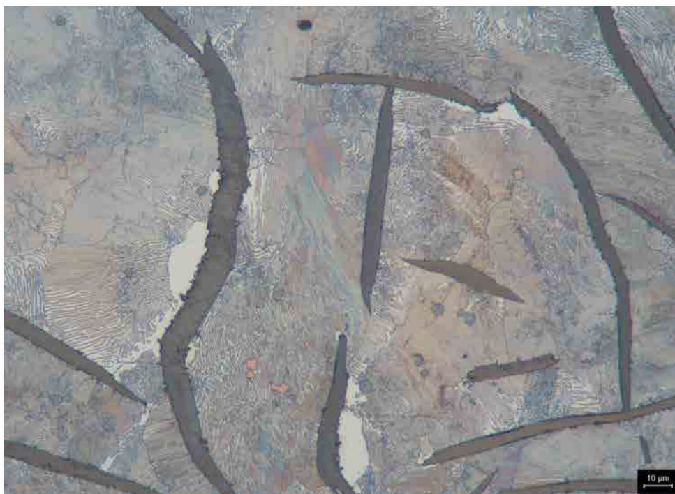
The microstructure of GJL after etching under the microscope (500:1)
