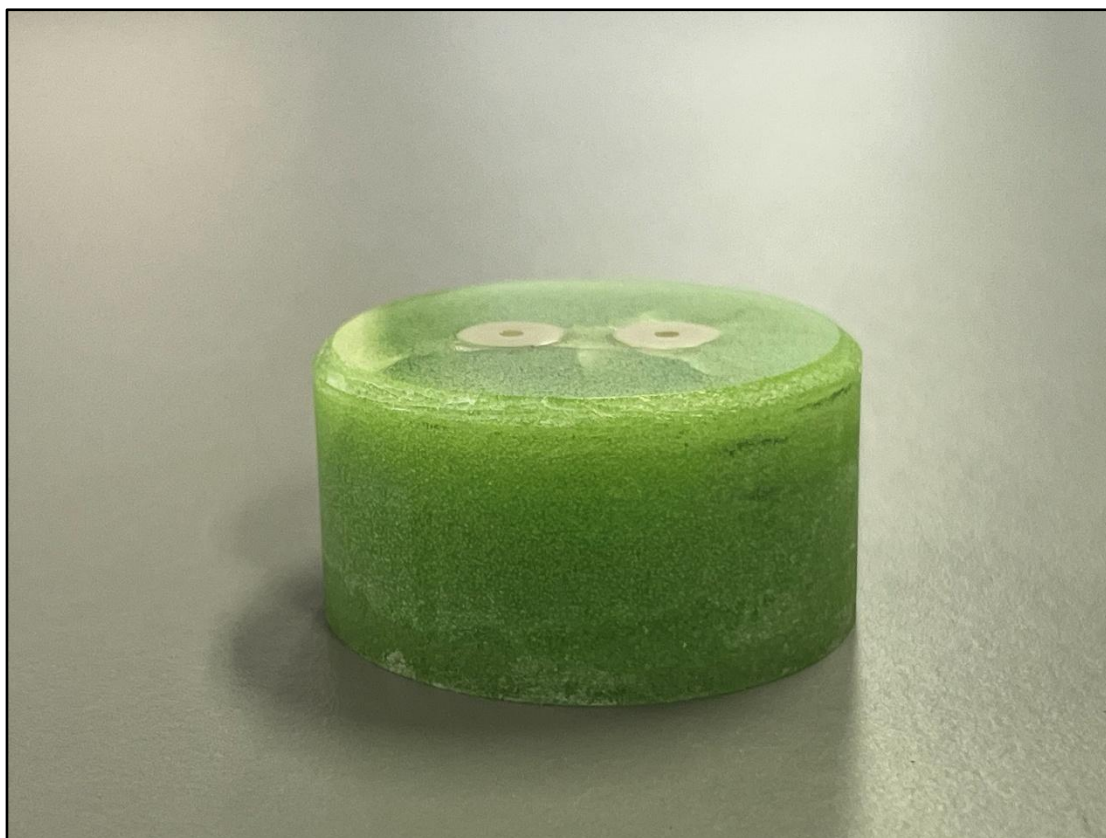
Figure 3. Overview of Coorstek-sample. The sample has a chamfer. The chamfer causes problems during sample leveling for the Qpol VIBRO.
