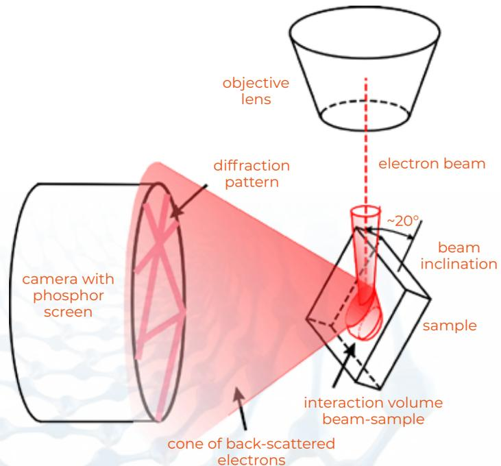
Figure 2: Setup of sample and detector within a scanning electron microscope (SEM).
