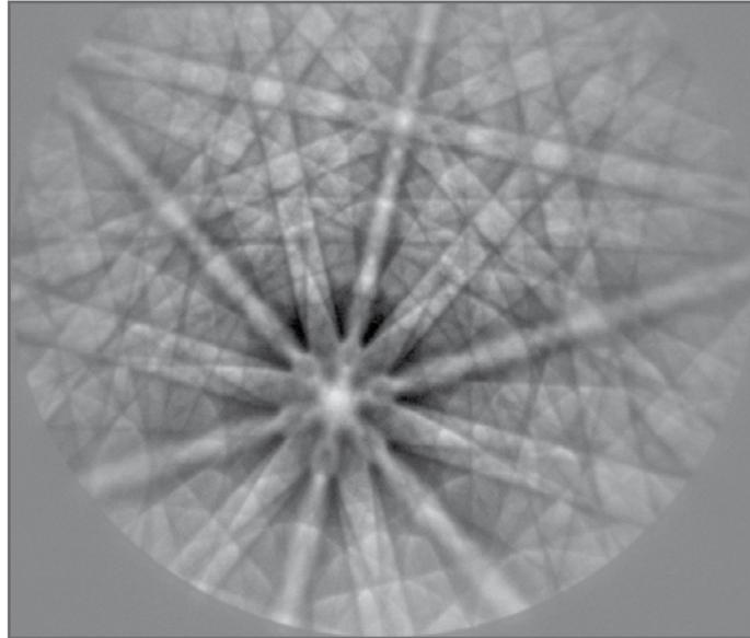
Figure 1: High-resolution EBSD pattern from an as-cast niobium sample (915 x 915 pixel). Exposure time 7 s, with background subtraction.
